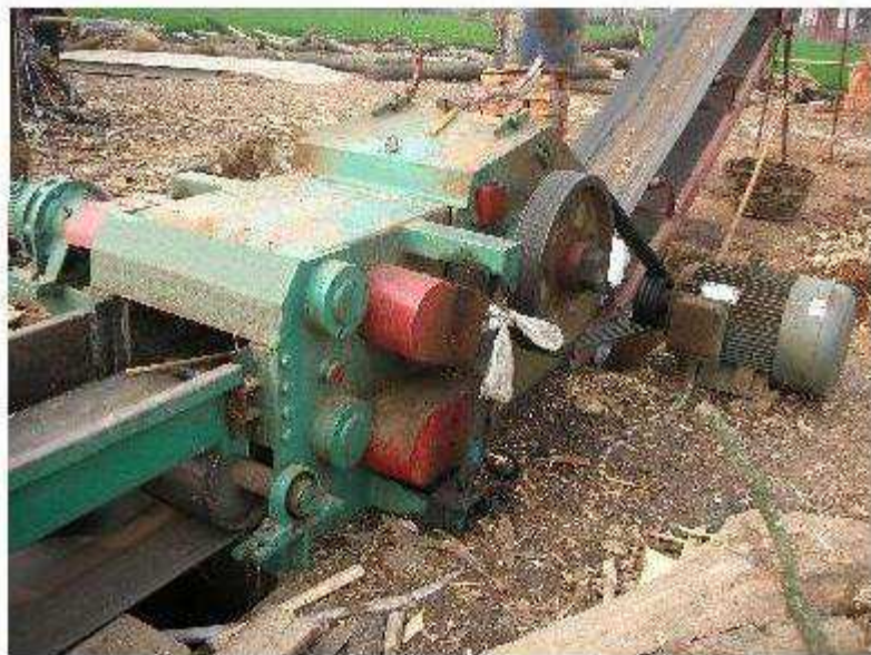
Wood crusher installed
